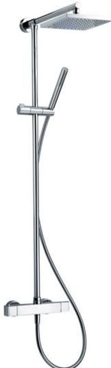
Thermostatic shower column, 2-functions, 2 outlet deviastop, not adjustable riser column, sliding handshower holder, D.26 mm ABS minimalist one spray handshower, 200x200 mm square showerhead, 150 cm smooth SUPREME Flexible Hose
