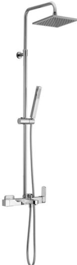
3-functions single lever bath set,2 outlet diverter,adjustable riser column,sliding shower bracket,ABS 27x27mm one spray minimalist square handshower,200x200 mm ABS square showerhead,150 cm smooth SILVERFLEX Flexible Hose
