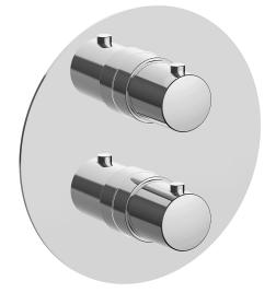
MODEL **SMOBT030** Exposed part for Thermostatic One Box Valve,wth 1-2-3 outlet deviastop,Minimum depth of installation: 67 mm,without concealed part,for items ZA00B030-ZA00B031
